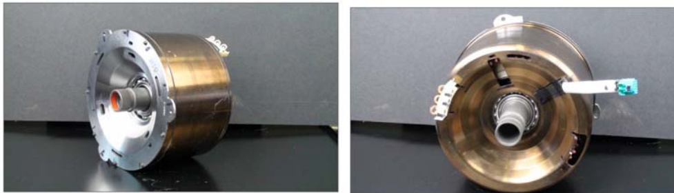
Figure 2. Drive Motor-Generator 2 nd Position
